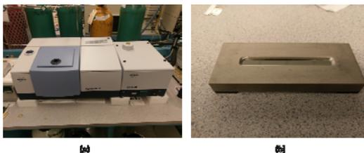
**FIGURE 1 FTIR-ATR (a) FTIR – Bruker Tensor 37, and (b) ATR boat device**
