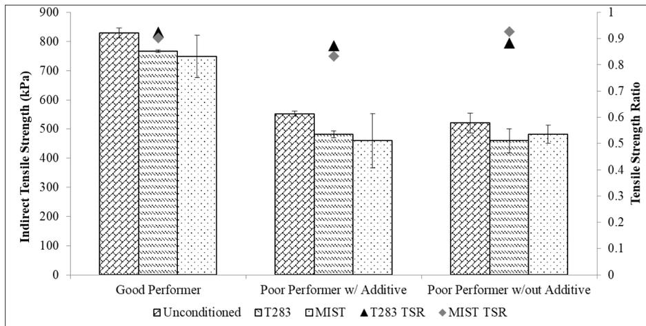
**FIGURE 1: Indirect Tensile Strength Results**
