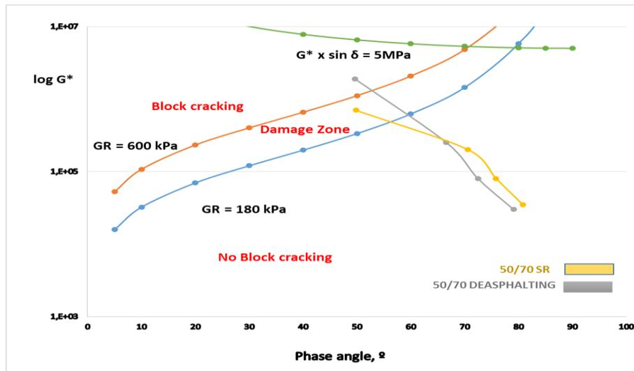
FIGURE 4 - Black Space Diagram of samples submitted to UV Suntest aging
