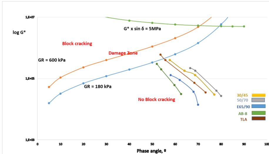
FIGURE 3 - Black Space Diagram of samples submitted to solar radiation aging
