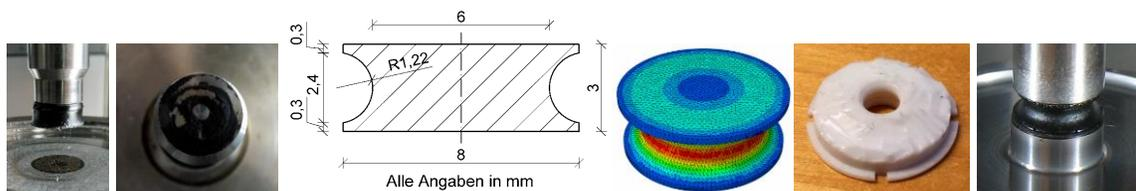
31 **FIGURE 2 Failure types, hyperboloid shape, FE model, silicone mould, alt. solution**
