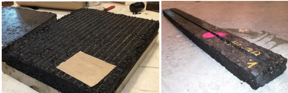
FIGURE 4 Prefabricated asphalt specimens with groove for FBGs embedment preparation
