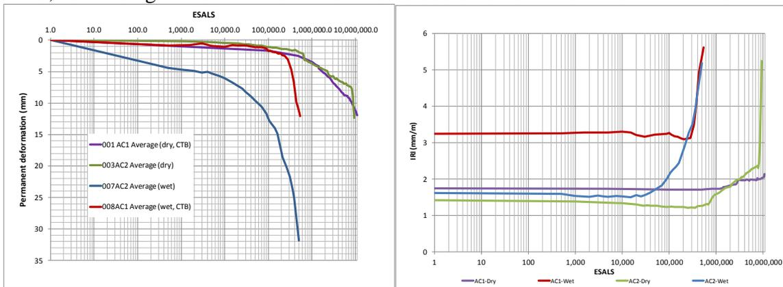
26 **Figure 6 and 7 Change in permanent deformation and Change in IRI**
