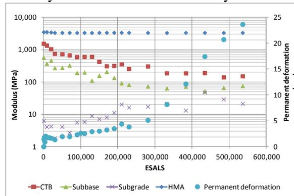
19 **Figure 5 Change in layer stiffness and permanent deformation for section AC1-Wet.**
