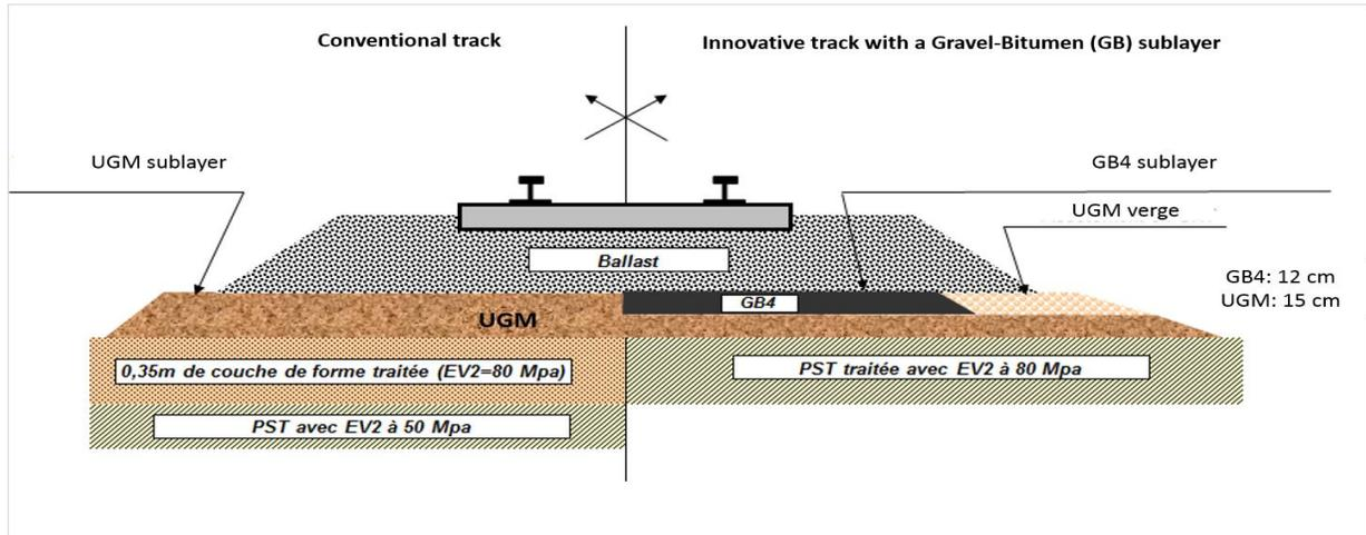
Figure 1- Different structure of the HSL BPL
