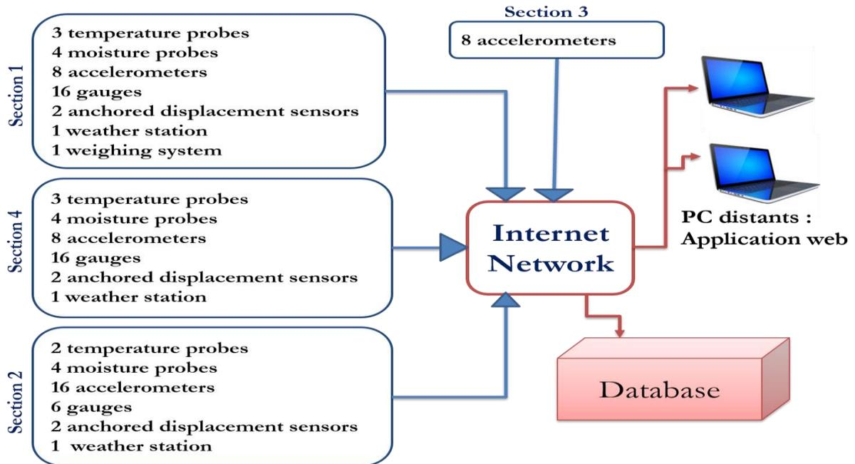
Figure 2 - Overall scheme of the instrumentation and acquisition system
