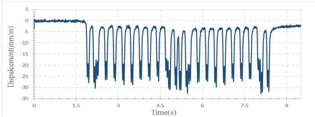
Figure 4 - Deflection signal of a double train passing on HSL BPL with V=217 Km/h
