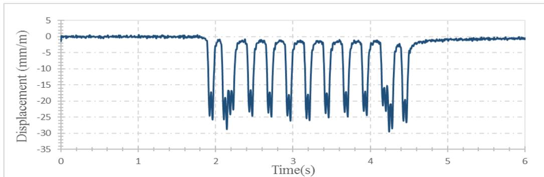
Figure 3 - Deflection signal of a simple train passing on HSL BPL with  $V=270$  Km/h
