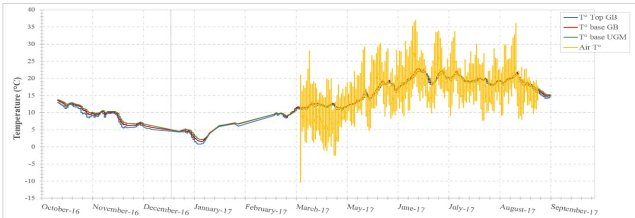
Figure 5 - Variation of sublayers and ambient air temperature in a section for 11 months period
