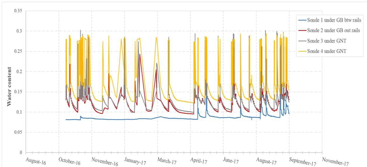
Figure 6 - Water content variation in a section with asphalt concrete for an 11months period
