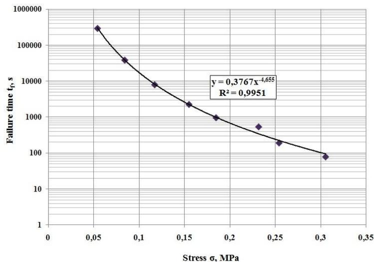
116 **FIGURE 6. Curve of Long-Term Strength for Asphalt Concrete**
