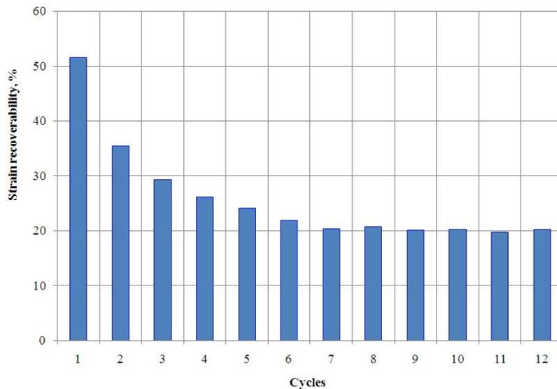
97 **FIGURE 5. Recoverability of Asphalt Concrete Strains in Cycles**
