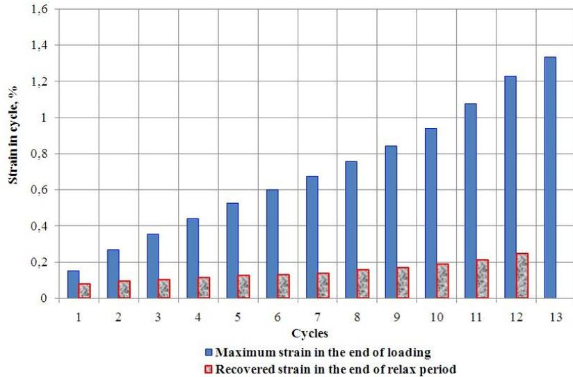
95 **FIGURE 4. Bar Charts of Maximum Strain of Asphalt Concrete in the End**
