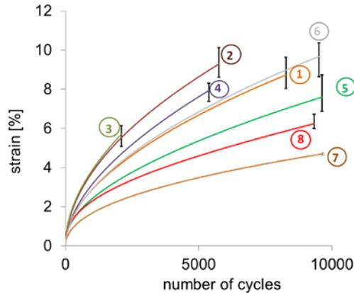
**FIGURE 2 Cyclic compression test results for all systems with scatter in terms of minimum and maximum values**
