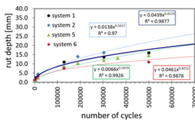
**FIGURE 4 Rutting test results for systems 1, 2, 5 and 6 (average of two profiles).**
