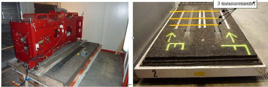
**FIGURE 3 Left: Model Mobile Load Simulator, right: 2 rutting profiles on system 5**
