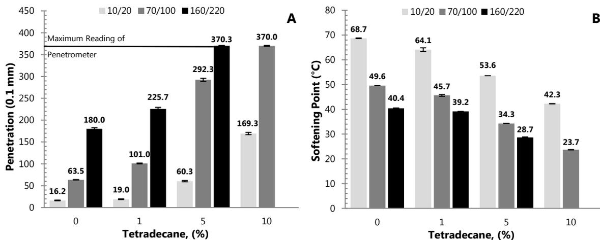
Figure 1: Effect of PCM modification on penetration (A) and softening point (B) of the different bitumens
