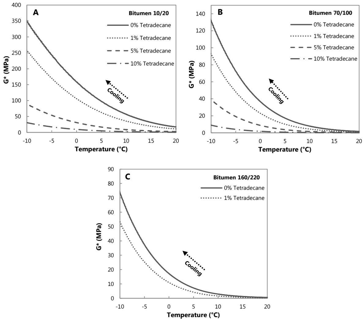
Figure 2: Effect of PCM modification on complex modulus as a function of temperature (Temperature sweep test)
