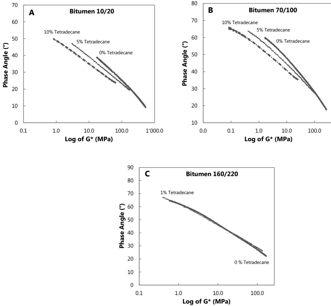
Figure 3: Effect of PCM modification on rheological parameters (Black curves)
