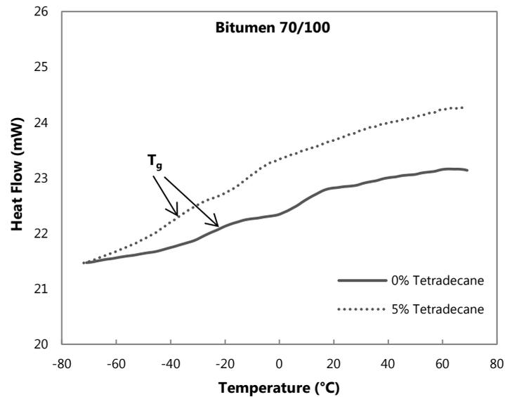
Figure 4: Thermal characterization of modified and unmodified bitumen with 5%. PCM (DSC Curves)
