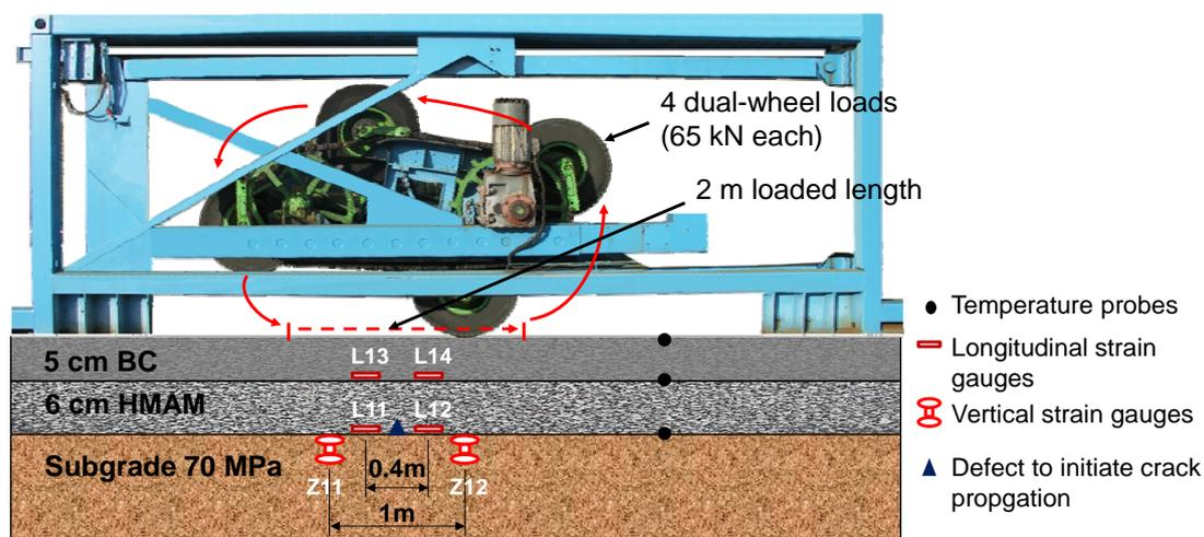
FIGURE 1 IFSTTAR's FABAC traffic simulator and the tested pavement structure
