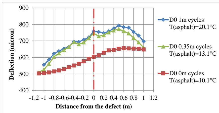
18 **FIGURE 5 Maximum deflections under the 65 kN FWD at every 0.1 m along the 2 m**
