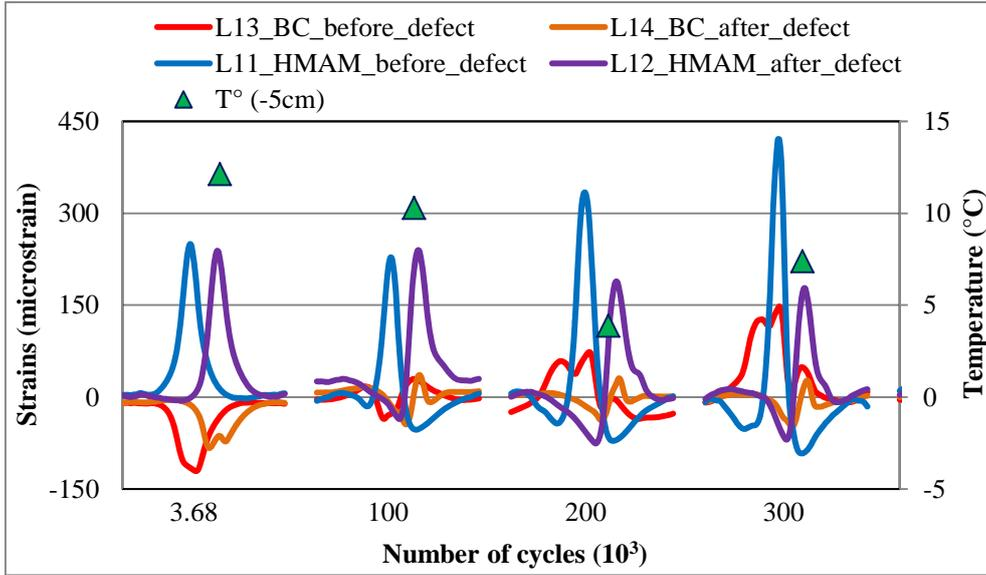
**FIGURE 2** Longitudinal strain profiles recorded by the gauges positioned in the asphalt layers at some selected numbers of repeated loading cycles
