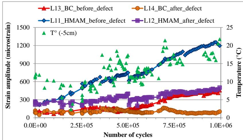
**FIGURE 3** Strain amplitudes in the asphalt layers measured all along the test
