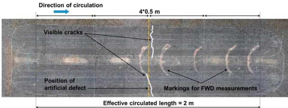
**FIGURE 4** Top view picture of the pavement section after 1 million loading cycles: close-up of wheel path
