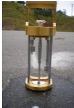
3 4 5 6 7 8 9 10 11 12 13 14 FIGURE 6 Outflow meter equipment photo. Source: ASTM
